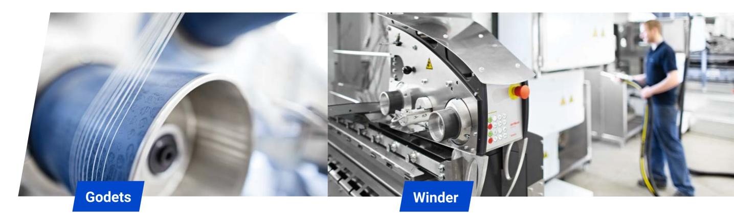
The induction-heated HF series godets have also been taken from the proven large-scale Oerlikon Barmag spinning systems.
