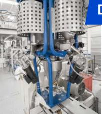
The gravimetric dosing and blending system grants high-precision dosing of masterbatches and additives down to  $0.5\,\mathrm{kg/h}$ . The system can be designed with up to seven components to support individual compound recipes. Each component uses continuous gravimetric blending (loss in weight principle) to achieve excellent dosing accuracy. Inclined screw feeders improve the metering accuracy and prevent undesired dribble effects.
