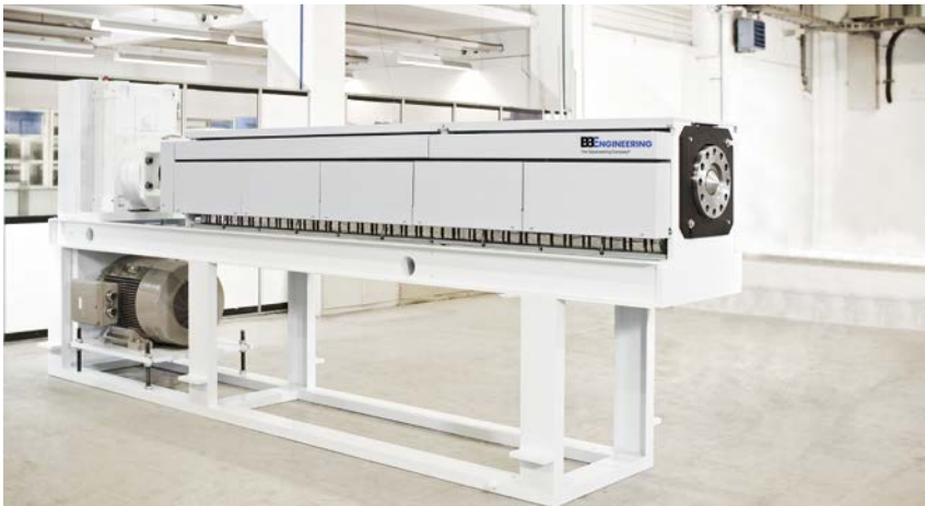
Design example: 30D extruder without degassing
